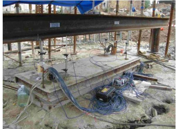
Figure 4 Barrette head under bi-directional static load testing
