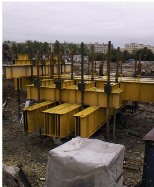
Figure 2 Reaction beam set-up for traditional 30 MN top down test
