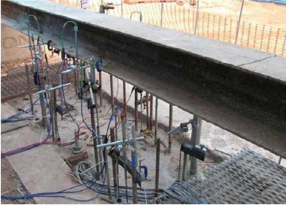
Figure 11.- Multilevel bi-directional testing set up at the barrette head. The beam provides reference only as the loading is applied internally to the structure
